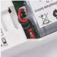
Self test & manual test switch
