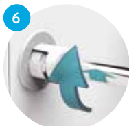
6 Rotate to apply pressure to activate the adhesive tape
